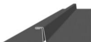
Angle standing seam joint
